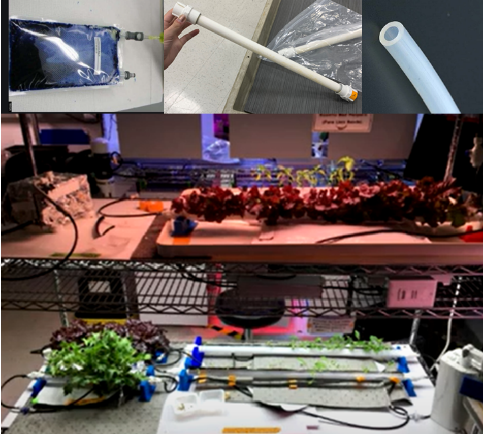
Figure 3: Top Left: Forward Osmosis Bag by HTI (Smith, 2011). Top Middle: KSC Porous Tube. Top right: Silicone Piping (Smith, 2011). Bottom: Fully set up PPTNDS in KSC Space Crop Production Laboratory (NASA Technology Transfer Program, 2020).
